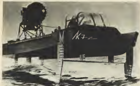
Experimental launch with automatically controlled underwater wings.
